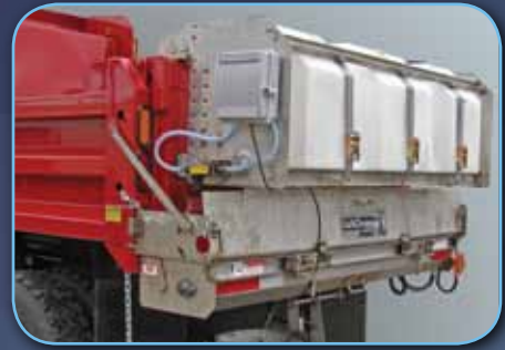
LS4T (tailgate mount 105 gal. poly reservoir)
