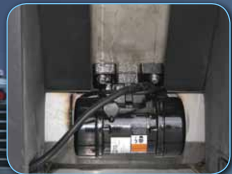
12 VDC vibrator rated at 400 force pounds
