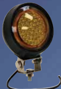
1492111 - 5" 12V-24V LED Utility Light Amber, 54 LED's, .3 Amps, 375 Lumens
