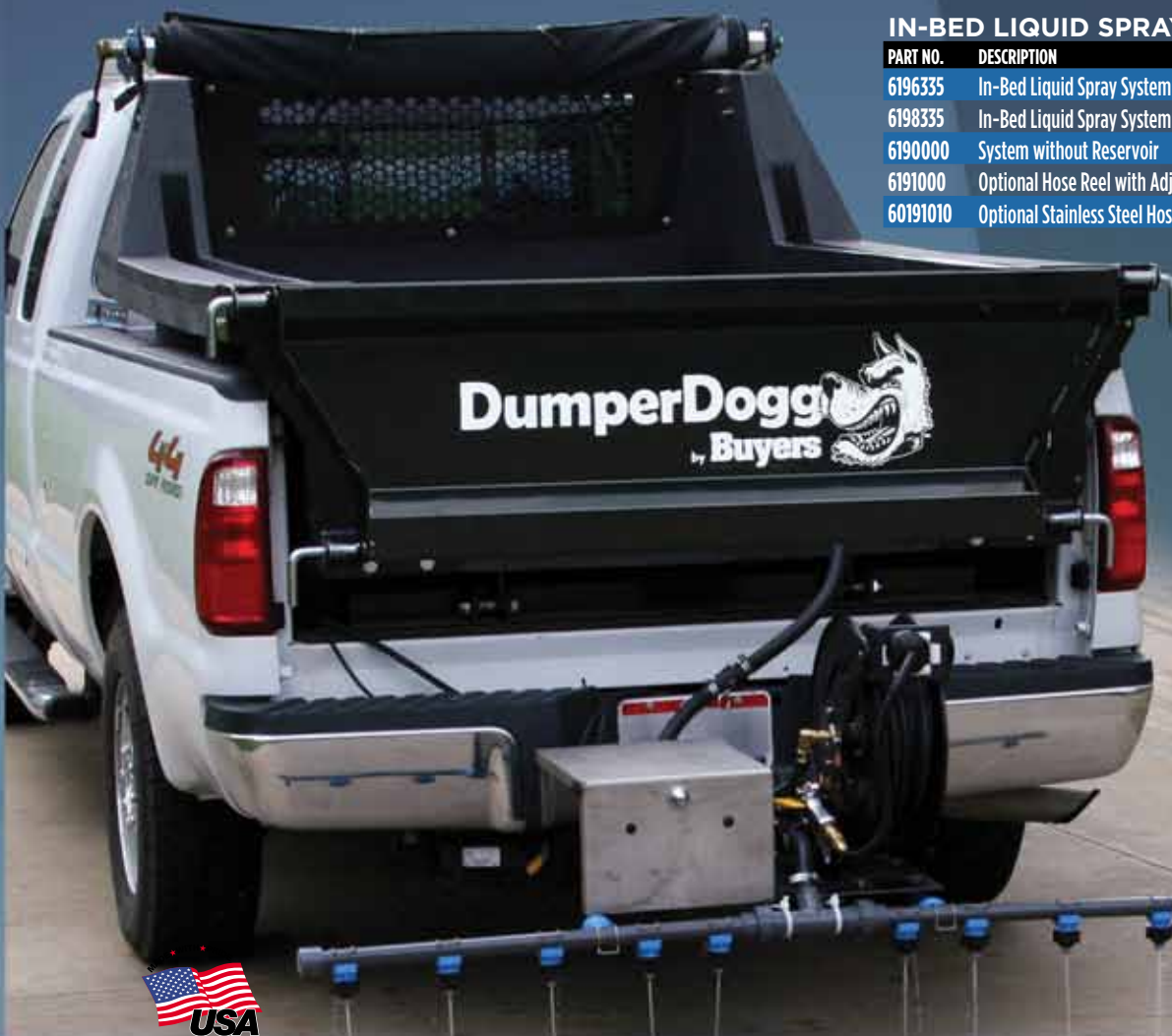
adjustable spray nozzle - pressure switch activates pump on demand
