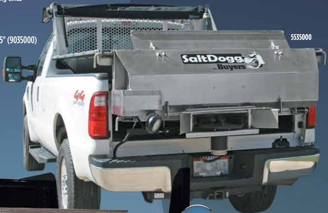
3016934 - Variable speed controller standard with 9035000 & 5535000
