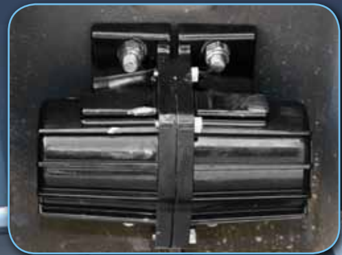
3020340 Optional Vibrator Shown Installed
