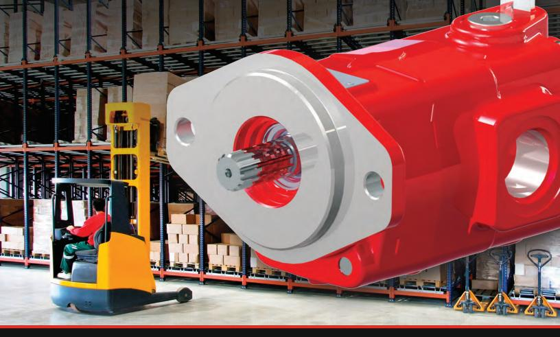
The "H"series utilizes a 3 port design; 1 inlet, a controlled flow port and a bypass/excess flow port. The internal flow control spool provides the desired amount of flow to the primary application via the controlled flow port regardless of pump speed or load demand changes.
