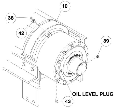
Install winch and connect pressure lines. Apply at least 230 PSI pressure to release brake and verify that brake releases, by observing that the winch drum rotates.
