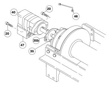
3. Remove brake assembly screws #16 from brake 35a to access (2) mounting screws #19 attaching brake adapter plate #35d to end bearing #9. CAUTION: BRAKE IS SPRING-LOADED BY CLUTCH SPRING AND MUST BE RESTRAINED AGAINST END BEARING AS MOUNTING SCREWS ARE REMOVED. Remove coupling #7 and gasket #35e from end bearing. Take note of mounting configuration for proper mounting of parts during reassembly.
