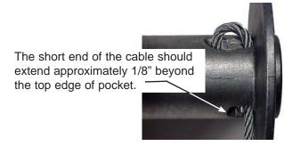
Wind on the cable by pulling in a light load to keep the tension constant. Allow the cable to swivel by using a length of chain or a swivel block between the cable hook and the load.
