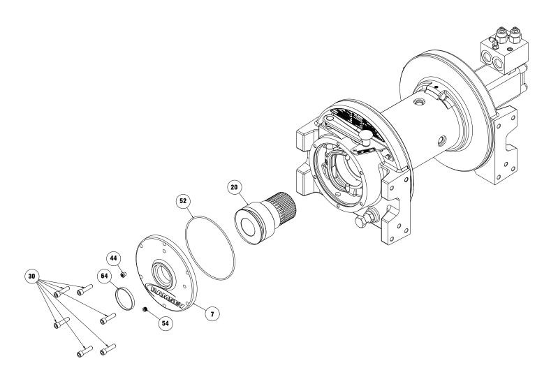
6. Slide clutch end bearing #2 from drum. Drum freespool drag puck #12, drum freespool spring #68, and brake disc spacer #73 will fall out when end bearing is removed from drum. Retain these items for re-assembly.
