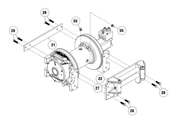
3. Position roller guide face down on a level surface and (2) capscrews #27 and roller guide tie bar #22. Horizontal rollers #37 can be removed from the left and right hand roller guides once the tie bar has been removed. Horizontal rollers #37 have (2) lube fittings #43, one located at either end of the roller.
