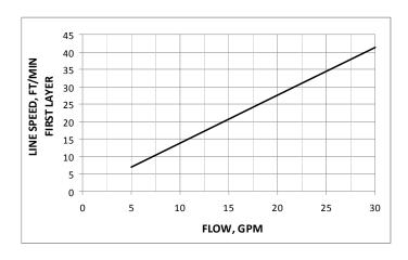
**BASED ON 14.9 CU IN/REV MOTOR**
