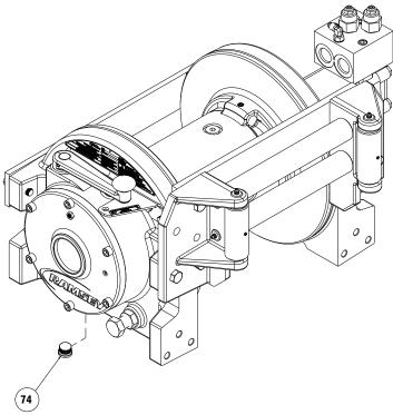
2. Freespool drum to locate drain hole in bottom. Remove plugs #55 from barrel of drum. Drain oil from drum barrel. Remove tie plate #21 by loosening (2) capscrews #28 each side. Loosen but do not remove (2) capscrews #27 on roller guide tie plate #22. Remove (4) capscrews #28 and roller guide.
