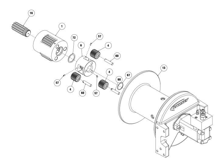
9. Remove drum #13 from motor end bearing #3. Remove drum seal #65. Check for signs of wear and replace if necessary.
