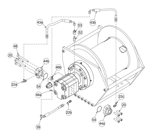
6. Remove (2) fittings #46a and #46b from counterbalance valve #41. Remove counterbalance valve #41by removing (2) bolts #47. The motor #24 can be removed by removing (4) bolts #50.
