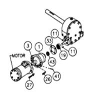
Place motor shaft, with key in keyway, into coupling. Secure motor to adapter, using two (2) capscrews #27 and lockwashers. TIGHTEN CAPSCREWS TO 75 FT. LBS. (102 Nm.) EACH.
