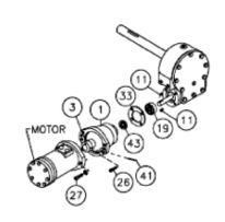
4. See page 12 for servicing the oil cooled brake. Remove brake housing mounting screws #25 and remove brake with gasket. Replace gasket #33. Remove worm #16 and bearings #19 from gear housing. Use soft hammer to gently tap input end of worm and drive worm and bearing from gear housing. Once worm has been removed from housing, bearing can be pressed from end of worm.
