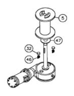
15. Slide spacer #48 over end of drum shaft. Press drum downward to compress drag brake springs in gear housing. Insert keys #35 into keyways with sharp edge of keys pointing outward and notched end of keys upward. A rubber or brass mallet will be needed to gently tap keys into position.
