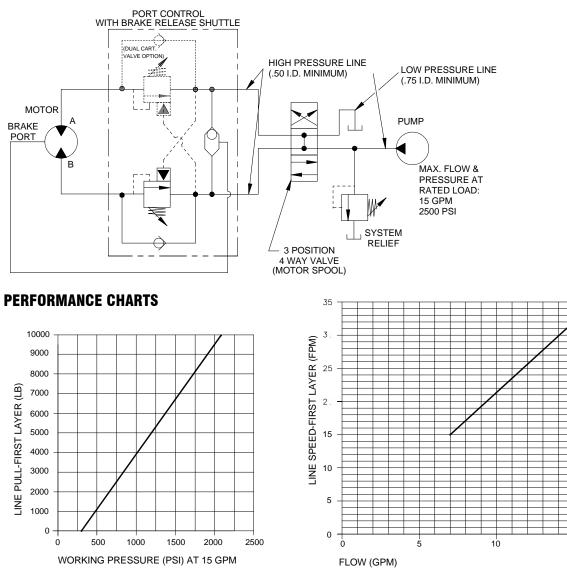
BASED ON 24.9 CU. IN. MOTOR
