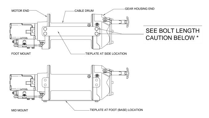
In the as-installed condition, if the winch is mid-mounted, then at least one tie-plate must be attached to the mounting feet at the bottom of the winch to maintain alignment. If the winch is foot mounted then at least one tie-plate must remain mounted at midpoint of winch to maintain alignment. It is always preferred to used BOTH tie-plates in the final installed configuration.
