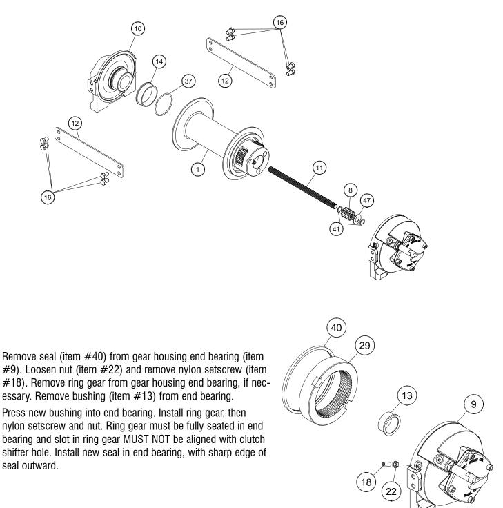
Generously apply grease (MOBILITH SHC 007) to teeth of ring gear (item #29), teeth of planet gears in drum (item #1), and to bushing (item #13) in gear housing end bearing. Apply a small amount of grease to base of bushing (item #14) on motor end bearing. Apply grease to teeth of output sun gear (item #8) and input shaft (item #11).
