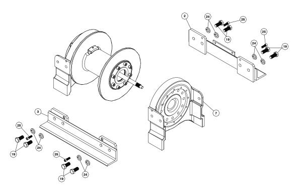
8. Pull drum assembly #1 from end bearing #6. Remove quad-rings #34 from grooves in drum bushings. Remove input shaft #11 and coupling #4from end bearing. Examine splined ends of input shaft for signs of wear, replace if damaged. Examine drum assembly #1 for signs of wear.
