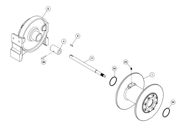
9. If splines inside drum driver #102 are damaged, drum driver must be replaced. Remove drum driver by unscrewing (8) capscrews #105. If bushings show signs of wear, replace by pressing old bushings from drum #101 and removing o-rings from grooves in drum and drum driver. Place well oiled o-rings #106 into driver and drum. Place well oiled o-ring #107 on outside of driver. Press bushings #104 into drum driver until flange is flush and #103 is flush against drum.
