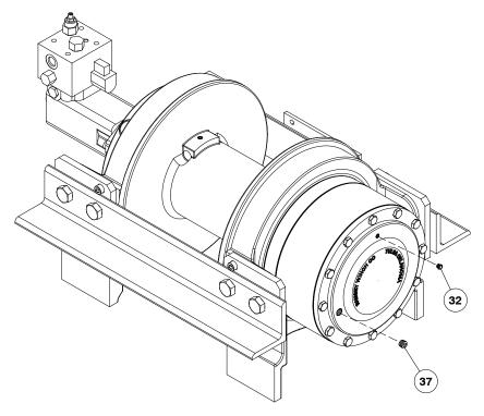
2. Disconnect tube #40 from elbow #43 on valve #41 and fitting #29 on brake #30b. Remove motor #33 and gasket #30a by removing (2) capscrews #22. Remove valve #41, if needed, from motor by loosening (4) capscrews #16.
