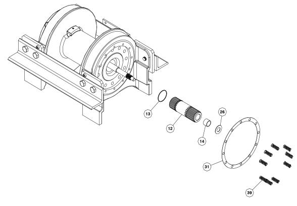
7. Remove winch tie bars #2 and #3 by removing (8) capscrews #19, (8) lock washers # 24, and (4) shoulder bolts #25. Pull gear end bearing #7 from drum assembly #1.
