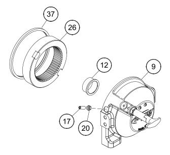
Generously apply grease (MOBILITH SHC 007) to teeth of ring gear (item #26), teeth of planet gears in drum (item #1), and to bushing (item #12) in gear housing end bearing. Apply a small amount of grease to base of bushing (item #13) on motor end bearing. Apply grease to teeth of output sun gear (item #7) and input shaft (item #10).
