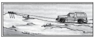
Stakes driven in solid earth and chained together make a good anchor point for self-recovery when no solid anchor point is available.
