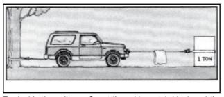
To double the pull, use 2-part line with snatch block and tie off to chassis. Take out of gear.
