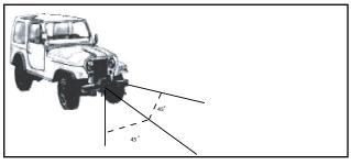
Winches equipped with cable guide fairleads can pull from several directions. Pull from an angle only to straighten up the vehicle-otherwise you can damage structural members or other parts of your vehicle and cause excess cable buildup on one end of the winch drum.
