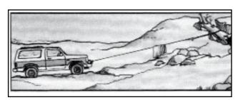
For a solid anchor, bury a log with earth or sand or place it in a deep ravine
