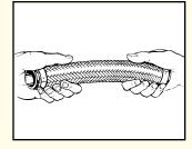
Step 2. Stretch until snug, mark length and cut with tin snips.
