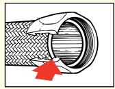
Step 2. Insert hose in socket with twisting, pushing motion until hose is in line with back of socket threads.
