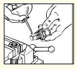
Step 4. Lubricate inside of hose and nipple threads liberally using S.A.E. 30 lubricating oil or Aeroquip FBM3553 Hose Assembly Lube.
