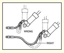
In applications where there is considerable vibration or flexing, allow additional hose length. Metal hose fittings, of course, are not flexible, and proper installation protects metal parts from undue stress and avoids kinks in the hose.
