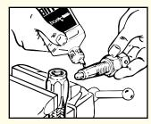
Step 3. Male Ends: Push assembly tool into nipple.
