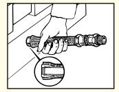
Step 2. Push the sleeve over the end of the tube and under the wire braid by hand. Complete positioning of the sleeve by pushing the hose end against a flat surface. Visually inspect to see that the tube butts against the inside shoulder of the sleeve. Set the sleeve barbs into the Teflon\* tube by pushing a round nose tapered punch into the end of the sleeve and tube.
