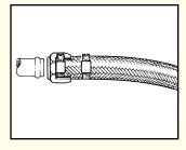
Step 2. Push cap (socket) onto hose until it bottoms. Then slide clamp under cap.
