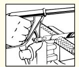
Step 1. Cut hose square with fine-tooth hacksaw or cut-off wheel.
