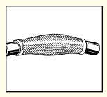
Step 1. Disconnect the radiator hose. Slide overbraid over the radiator hose.
