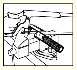
Step 1. Cut hose square to length with fine-tooth hack saw or cut-off wheel. To minimize wire braid flare out, wrap hose with masking tape and cut through tape. Remove tape, trim loose wires and flush with lube before next step. Burrs on bore of tube should be removed with a knife. Clean the hose bore.
