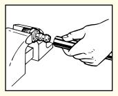
Step 2. Push hose on fitting until hose end bottoms underneath protective cap as shown. Clean, proof test to twice operating pressure and inspect all assemblies.
