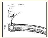
Step 3. Push assembly onto beaded tube. Position clamp for appearance. Tighten with a screwdriver.
