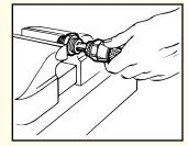
Step 3. Lubricate nipple and socket threads. Use a molydisulfide base lubricant for stainless steel fittings (e.g. Molykote Type G); lubricants containing chloride are not recommended. Other material combinations use standard petroleum lubricants. Hold the nipple with hex in the vise. Push hose over nipple with twisting motion until seated against nipple chamfer. Push socket forward and start threading of socket to nipple.
