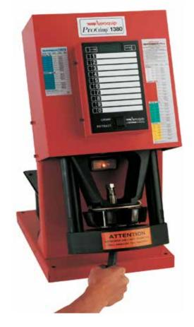
The ProCrimp® 1380 is totally compatible with Eaton's MatchMate® Plus hose assembly program. Matching and mating hose to fittings and to the tooling in the ProCrimp® 1380 make hose assembly simpler than ever. Decals have been prepared to fit the ProCrimp® 1380 with all of the MatchMate Plus hose styles, including MatchMate BLUE®
