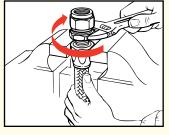
Step 6. Complete assembly using wrench while continuing to hold hose in position. Maximum allowable gap is .031 inches. Your thumbnail is a convenient measuring device.
