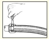
Step 3. Reconnect radiator hose and secure hose and overbraid with clamp or ProClamp clamp.
