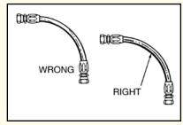
If a hose is installed with a twist in it, operating pressures tend to force it straight. This can loosen the fitting nut. Twisting can cause reinforcement separation, and the hose could burst at the point of strain.
