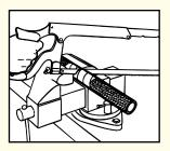
Step 1. Cut hose square to length with fine-tooth hack saw or cut-off wheel. To minimize wire braid flare out, wrap hose with masking tape and cut through tape. Remove tape before next step.
