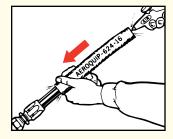
Step 1. Follow the appropriate hose assembly instructions through the assembly of one end fitting. Cut firesleeve to same length as hose. Start firesleeve over cut end of hose.
