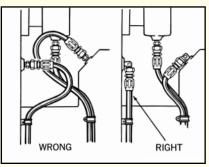
When 90° adapters were used, this assembly became neater-looking and easier to inspect and maintain. It uses less hose, too!
