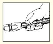
Step 7. Important—Check hose for pushout by observing hose position mark. Pushout should not be evident. CLEAN, PROOF TEST TO TWICE OPERATING PRESSURE AND INSPECT ALL ASSEMBLIES. Disassemble in reverse order.
