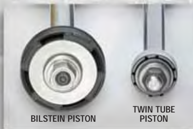
Gas pressure shock, no foaming
